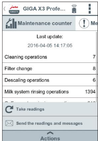
Fig. 31: Selection of actions for maintenance counter
