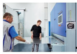
First, the surface of the blank aluminum panels are given their characteristic texture and tactile quality by means of grinding and brushing.
