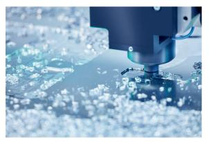
A modern CNC machine mills the required shapes and bevel designs from the aluminum panel with the utmost precision.
